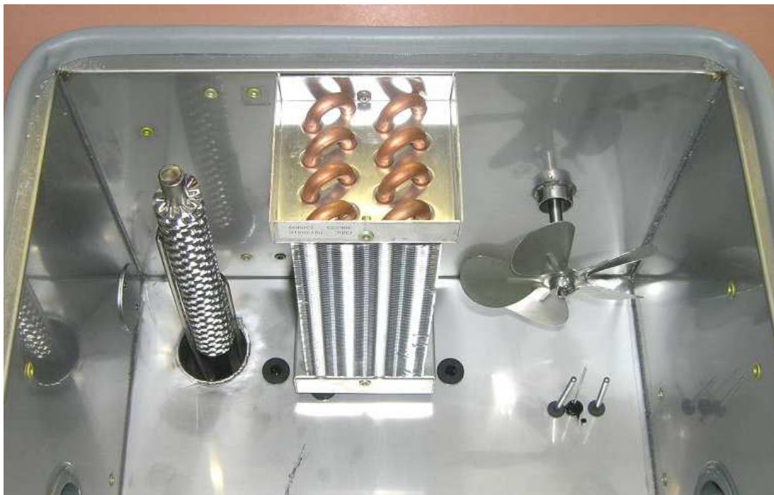
Figure 17 Conditioning Plenum Model TJR-INS
